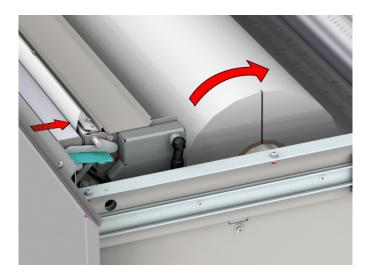
4. If necessary, you can manually cut the leading edge of the media when it has not been cut straight. Take a knife and cut the media in the cutting guide.
