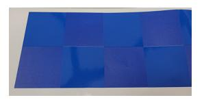
The misalignment is visible as white lines between the gloss and matte parts of the print.
