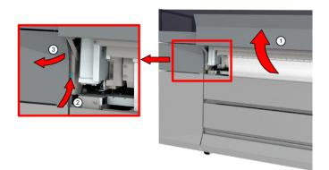
5. Open the manual maintenance door (3). A light is switched on.
