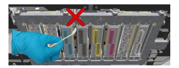
**9.** Dampen a new swab with cleaner MB and clean the outer edge of the matrix plate until all visible residue ink is gone.
