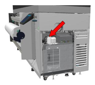
**11.** Pour one liter of demineralized water from the bottle in the pouring can.
