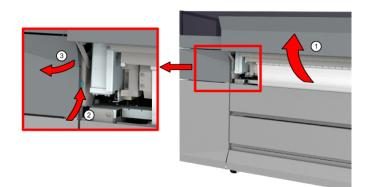
5. Open the manual maintenance door (3). A light is switched on.
