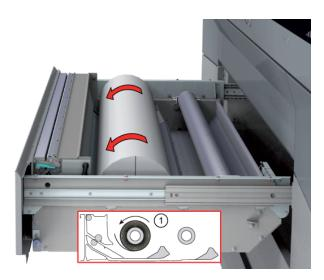
**11.** Use both hands to move the media forward and slide it under the metal paper guide (2) until the media is transported automatically. You will hear a beeping sound when the media is correctly fed and loaded.
