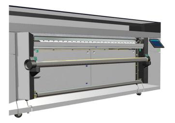
**2.** Push the green levers on both sides of the take-up media shaft. Remove the take-up media shaft from the winder.
